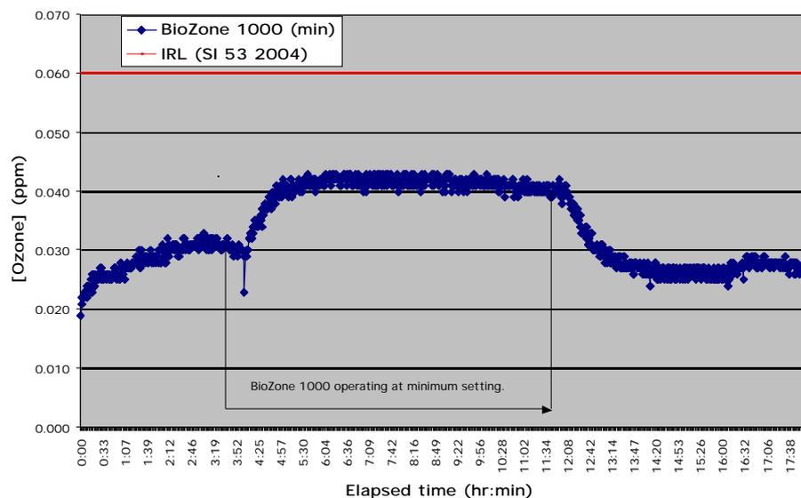
**Figure 1.** Ozone concentrations measured in a passively-ventilated seminar room before, during and after operation of a BioZone 1000 air purifier at minimum setting. The operational details are given in Methods 3.1.2.1. (run-protocol A).
