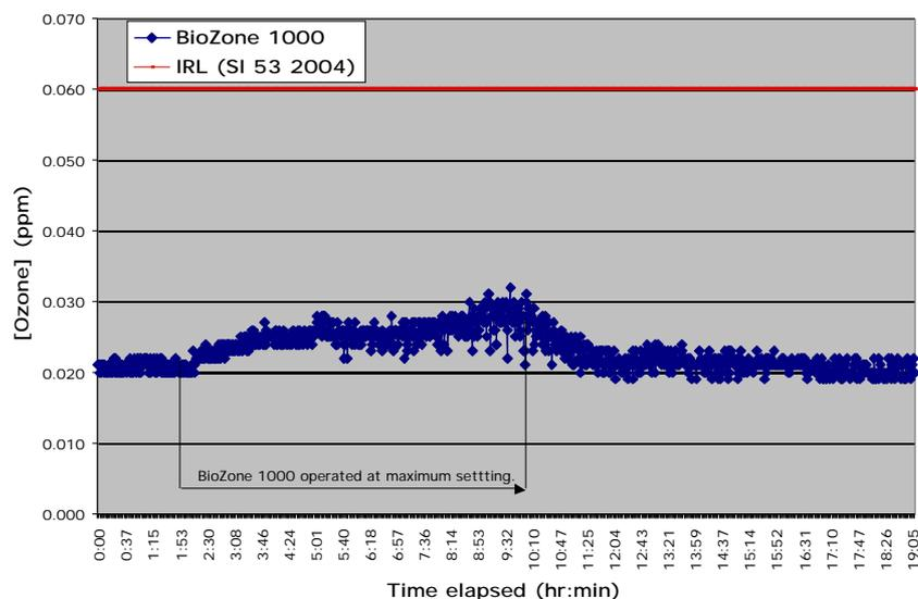
**Figure 3.** Ozone concentrations measured in a passively-ventilated seminar room before, during and after operation of a BioZone 1000 air purifier at maximum setting. The operational details are given in Methods 3.1.2.1. (run-protocol C).
