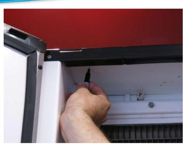
The proper spacing will prevent the return tube from interfering with the ice curtain operation
