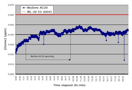
**Figure 4.** Ozone concentrations measured in a passively-ventilated toilet before, during and after operation of a BioZone AC20 air purifier. The operational details are given in Methods 3.1.2.2.
