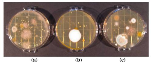
Figure 7. Cassettes incubated at 37 °C for 48 hours for air samples taken in a seminar room (Series 2): sample taken (a) prior to a three-hour BioZone 1000 run; (b) after three hours, i.e. at the end of the run; (c) two hours after the run. Experimental details are given in the text.
