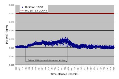
**Figure 3.** Ozone concentrations measured in a passively-ventilated seminar room before, during and after operation of a BioZone 1000 air purifier at maximum setting. The operational details are given in Methods 3.1.2.1. (runprotocol C).
