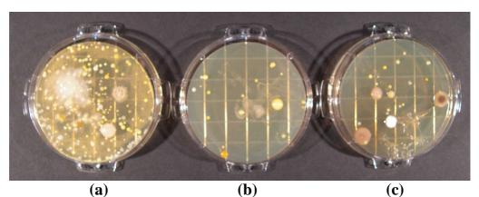
Figure 5. Cassettes incubated at 37 °C for 48 hours for air samples taken in a sealed room (Series 1): sample taken (a) prior to an 18-hour PowerZone-II run; (b) after a further one-hour operation of an aircirculation fan; (c) two days after the PowerZone run. Experimental details are given in the text.
