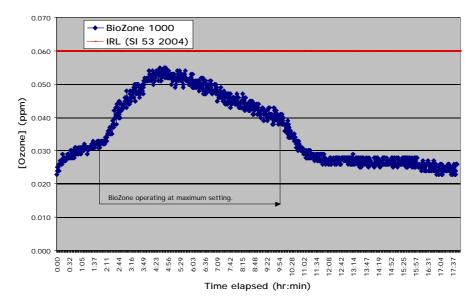
**Figure 2.** Ozone concentrations measured in a passively-ventilated seminar room before, during and after operation of a BioZone 1000 air purifier at maximum setting. The operational details are given in Methods 3.1.2.1. (run-protocol B).
