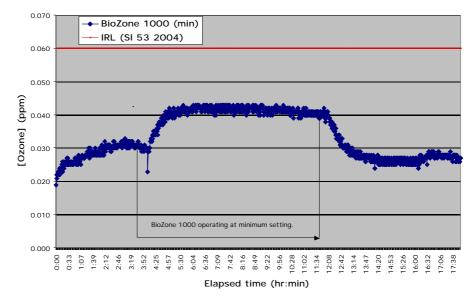
**Figure 1.** Ozone concentrations measured in a passively-ventilated seminar room before, during and after operation of a BioZone 1000 air purifier at minimum setting. The operational details are given in Methods 3.1.2.1. (run-protocol A).
