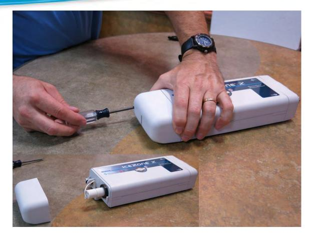
Remove the Input/Output cover from the IceZone<sup>®</sup> unit.
