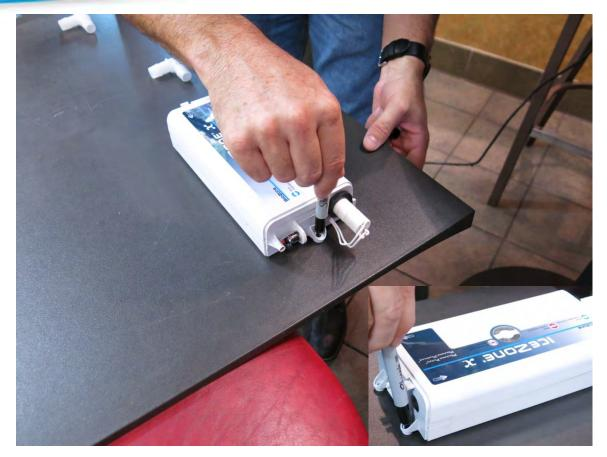
Drill the holes to mount the IceZone<sup>®</sup> Unit on the lid.
