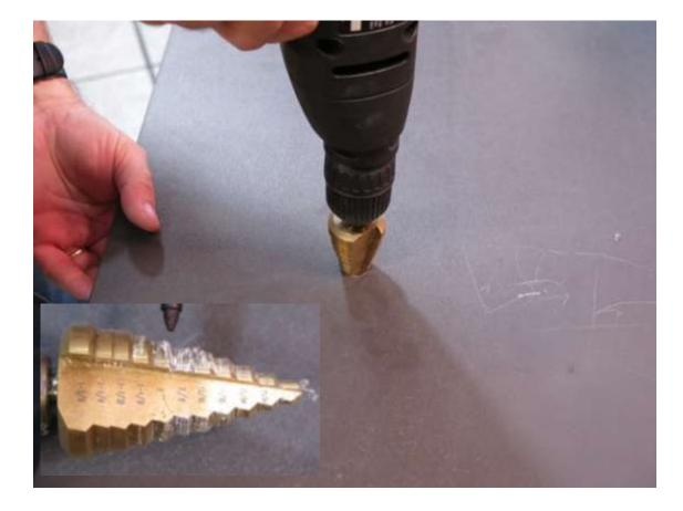
Clean the burrs from the hole edges and prepare to install the fittings.
