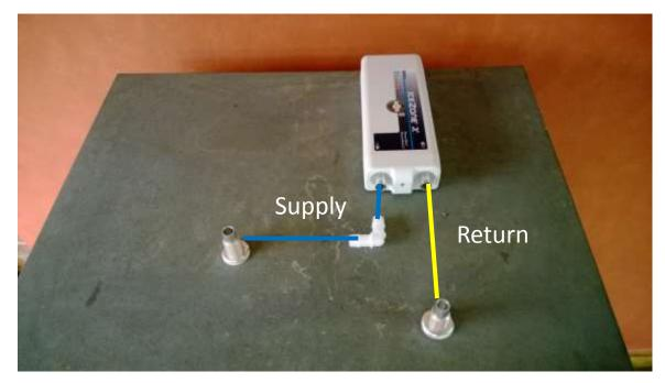
Mark the holes to mount the IceZone<sup>®</sup> Unit on the lid.
