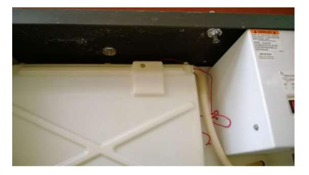
Install the remaining 12 inch length of tubing onto the return fitting.
