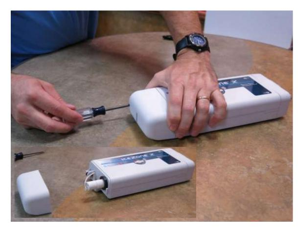
Remove the Input/Output cover from the IceZone<sup>®</sup> unit.
