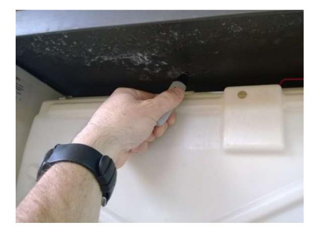
Mark the location for the IceZone<sup>®</sup> return fitting. This is the fitting where the plasma will return to the IceZone<sup>®</sup>. This should be located on the right side of the top cover (*looking at* the front of the ice *machine*). This hole should be spaced off of the interior wall of the ice machine by 2.0 inches. The hole should be spaced from the front edge of the ice machine cover by 2.0 inches also.
