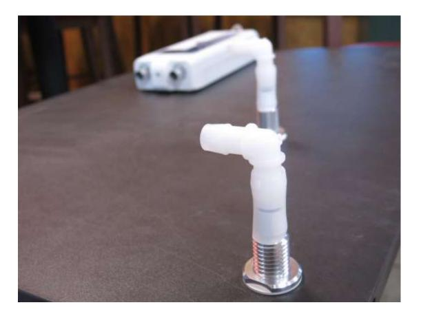
Cut and assemble the remaining supply and return tubing and fittings. There should be >12" of unused tubing.
