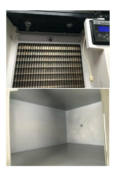
The machine and all removable parts were cleaned with hot water and detergent
